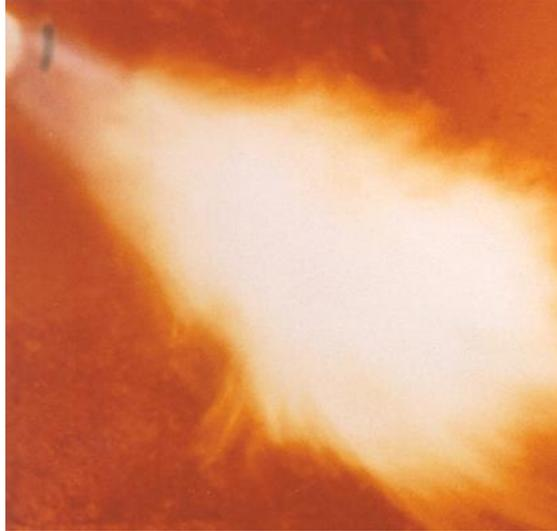
**Figure 10: A Hydrogen Flame Made Visible with the Addition of a Small Amount of Hydrocarbons**
